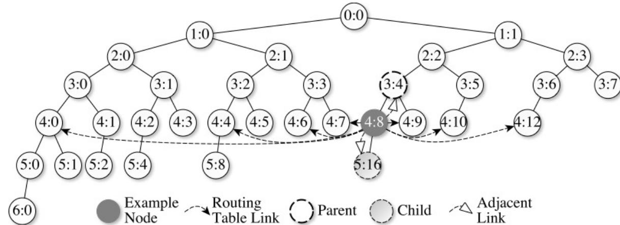
Figure 3: The BATON\* tree has a height of 7. Since node (4:8) has links to neighbors (4:0) and (4:4), links to the children are (5:0), (5:1), (5:8).
