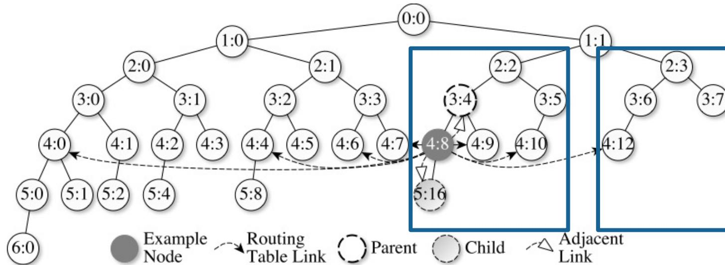
Figure 2: The BATON\* tree has a height of 7. Since node (4:8) has links to neighbors (4:0) and (4:4), links to the children are (5:0), (5:1), (5:8)
